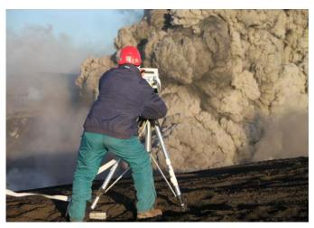
FTIR remote sensing of magma degassing from Eyjafjallajökull crater rim in May 2010, Iceland
